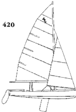
Length: 13'9" Board Type: centerboard Beam: 5'5" Weight: 220 lbs. Draft: 3'2" Self Rescuing: yes Sailors: 2 adults or 2-3 youths
