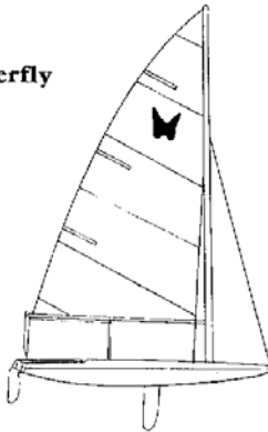
Length: 12'2" Board Type: daggerboard Beam: 4'6" Weight: 170 lbs. Draft: 2'6" Self Rescuing: yes Sailors: 1 adult or 1-2 youths
