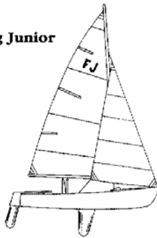
Length: 13'3" Board Type: centerboard Beam: 5'3" Weight: 209 lbs. Draft: 2'6" Self Rescuing: yes Sailors: 2 adults or 2-3 youths
