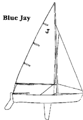
Blue Jay Length: 13'6" Board Type: centerboard Beam: 5'2" Weight: 275 lbs. Draft: 3'9" Self Rescuing: yes Sailors: 2 adults or 2-3 youths
